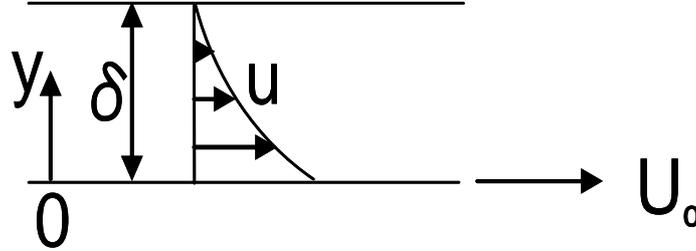
**Figure A1:** A definition sketch of flow between two parallel flat walls, one of which is at rest, the other is suddenly accelerated from the rest to a constant velocity  $U_0$ .
